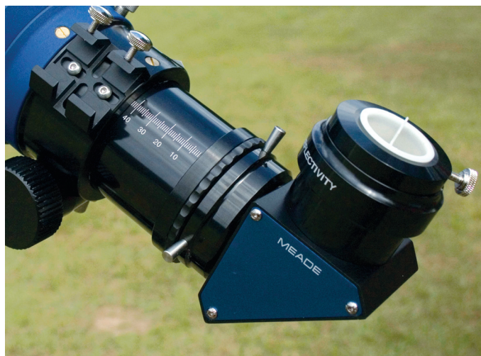
▲ Left: The beefy 3-inch focuser included with the 115 ED includes a blue anodized 10-to-1 fine-focus knob. Right: The unit’s drawtube is marked in centimeters to help quickly repeat focus with your favorite eyepieces and other accessories. The 2½- to 2-inch visual back can be independently rotated by holding the large knurled ring and turning the “captain’s wheel” with aluminum pegs.
