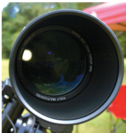
▲ The telescope’s 4½-inch triplet objective showed reflections only under bright sunlight.
