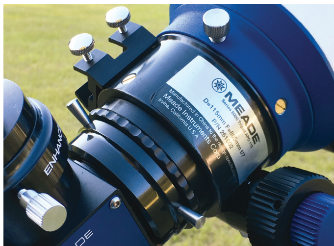
▲ Left: The beefy 3-inch focuser included with the 115 ED includes a blue anodized 10-to-1 fine-focus knob. Right: The unit’s drawtube is marked in centimeters to help quickly repeat focus with your favorite eyepieces and other accessories. The 2½- to 2-inch visual back can be independently rotated by holding the large knurled ring and turning the “captain’s wheel” with aluminum pegs.
