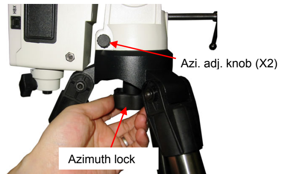
Figure 4. Install mount onto the tripod
